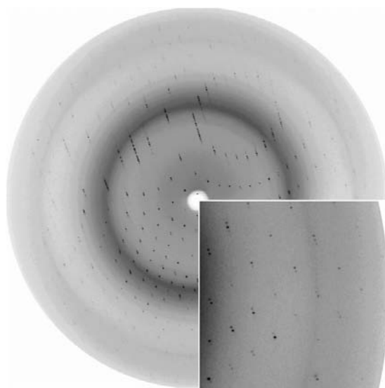
Figure 3 Diffraction image from a GlcV form A crystal collected using a 0.5^\circ oscillation and a 10 s exposure on a MAR 345 mm image-plate detector (beamline I711, Maxlab, Lund). The resolution at the edge of the detector is 1.9 \text{\AA} .
